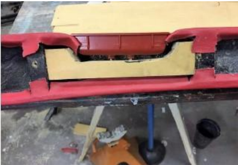
Back side of armrest with homemade stiffener installed for finger pocket to screw into.
