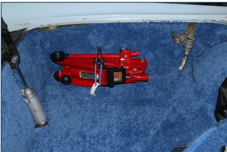
Bungee cords used to hold jack up so it stays out of the way when the top is down.
