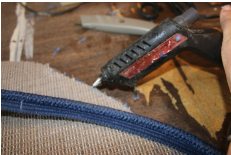
Hot glue gun is used to attach edge binding to carpet
