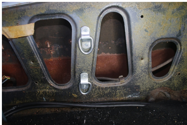
D-rings installed with carpet slots to permit exposure
