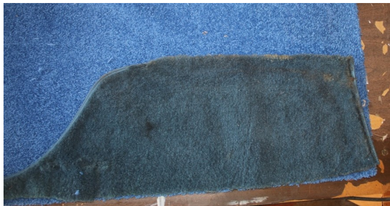
Old carpet used as template with adjustments as needed
