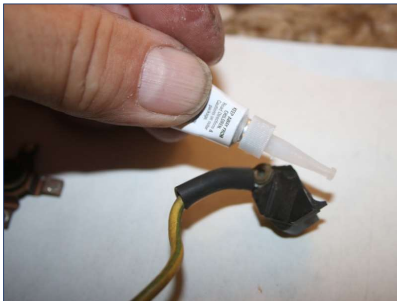
Use 'single use' glue tube to repair the connector block. Careful to avoid getting super-glue on your fingers
