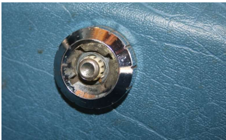
The problem is that the switch knob has been crushed into the switch
