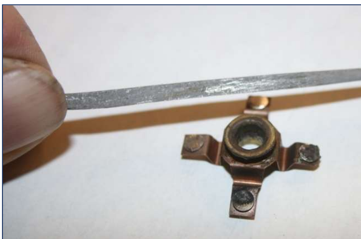
File off the accumulated crud on each contact point
