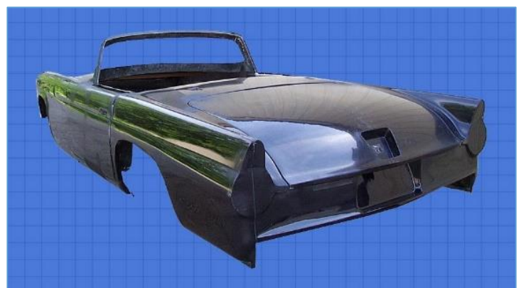
Brand-New, Hand-Laminated Fiberglass Outer Body Package includes a one-piece Main Body with Outer Doors, Outer Hood and Outer Trunk Lid.
