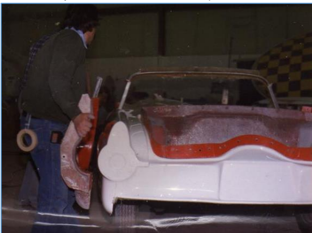
Molds being taken off the freshly built body at Sweet Reproductions.
