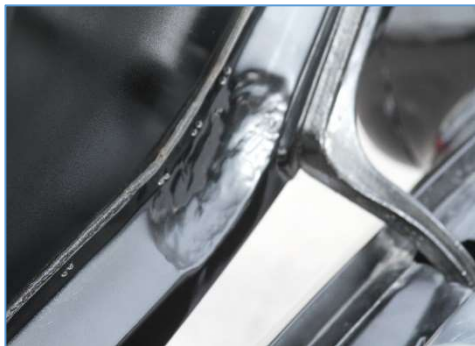
Hammered hand fitted interior hood strut, designed before computer aided design
